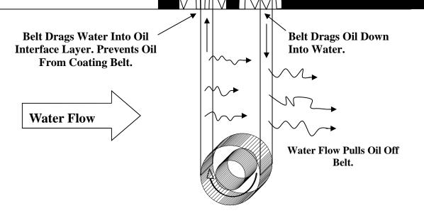
Free-floating oil and grease is reintroduced to water or coolant by Belt Skimmer. Water flow pulls oil off Belt and into metal working machines, rolling mills, filters and pumps. Oil reintroduced to water or coolant increases oil concentration levels which can increase oil & grease discharge levels, bacterial growth, water treatment costs and reduce product quality.
